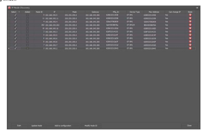
6. The adding process will take a while, and the software will check the state of all devices and a window will show, the "Added" be ticked means the device is already exist in the setting window, and with the state will be change to and click on "Close" button or "X" to exit discovery
