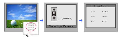
When Door Station is in standby, press '#' key
