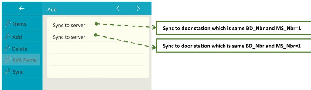
**Sync to server**, monitor will generate a monitoring list, and sync to door station DS1.
