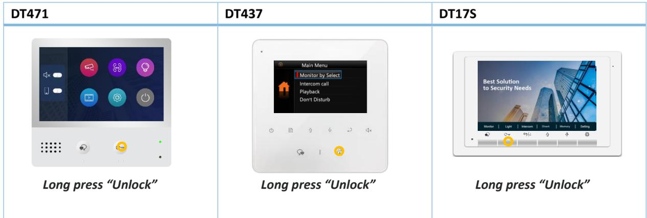
After, monitor will get calls from door station, as a simulator call, in the meantime, button door station’s button LED will flash.
